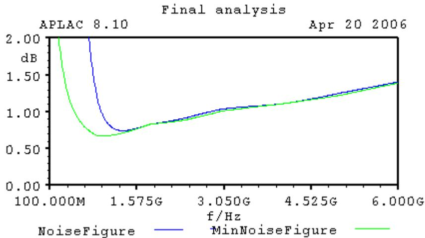
One can see that the circuit was optimised for about 1.3 GHz work.
