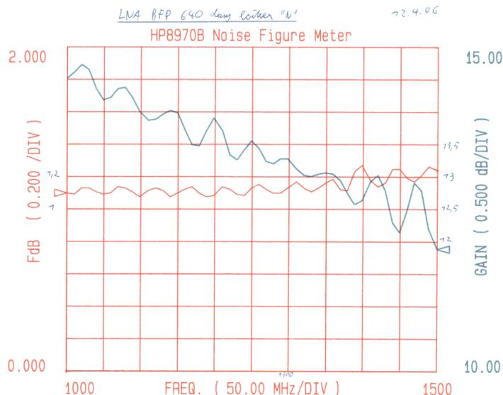
Be careful to the scaling of the graph. (0.2 dB/ division for NF ; 0.5 dB/ div for the gain, beginning at 10 dB)
