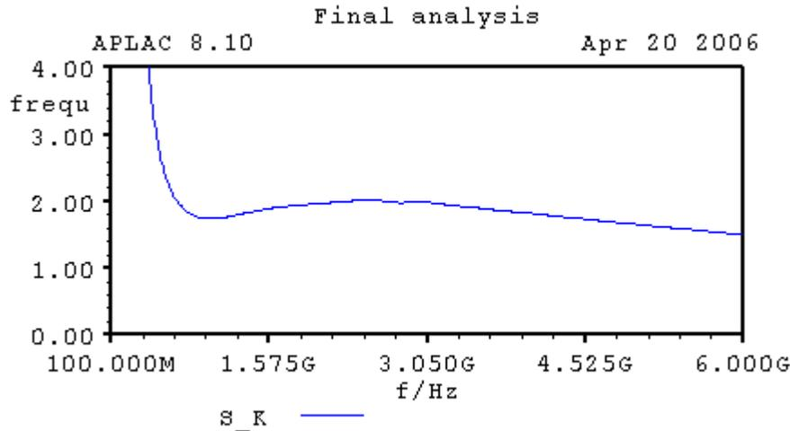
The graph shows the simulated Rollet stability factor (K factor). If this factor is greater than 1, the amplifier is stable. (there are some other conditions, but not leading to a problem here) The transistor's S parameters are given up to 6 GHz. That's the reason why the K factor was studied up to this limit. It is clear that  $K > 1$  is assured. It's good to have some margin as it's only a simulation! The real life will always be worse!
